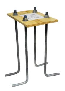
Strong Poles' pre-engineered Anchor Basket makes installations much faster, and alignment much easier. Simply push the Anchor Basket down into the wet concrete until the template is flush with the top of the concrete, and be sure that the conduit rises well above the hole in the template. Then, after the concrete has cured, remove the template and you are ready to mount the pole.
