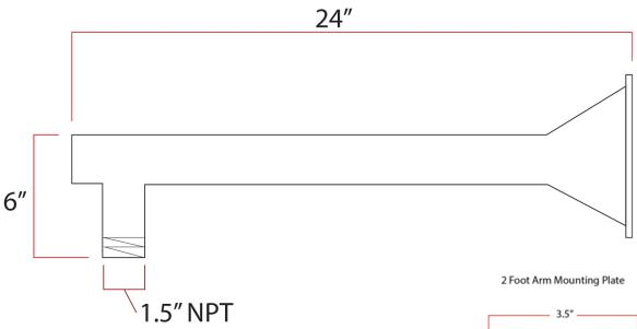
This arm takes your cameras and attachments out to 2 feet from the pole or wall. It can be added to any 4" Square Pole, or to any SteadyMax Pole with a Pedestal Mount or mounted directly to a wall.
