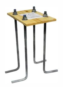
Strong Poles' pre-engineered Anchor Basket makes installations much faster, and alignment much easier. Simply push the Anchor Basket down into the wet concrete until the template is flush with the top of the concrete, and be sure that the conduit rises well above the hole in the template. Then before the concrete is cured, Removed the template and make sure foundation is level and smooth to mount the pole.
