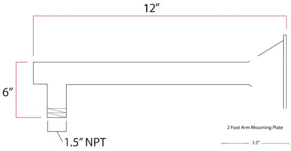
This arm takes your cameras and attachments out to 1 feet from the pole or wall. It can be added to any 4" Square Pole, or to any SteadyMax Pole with a Pedestal Mount or mounted directly to a wall.
